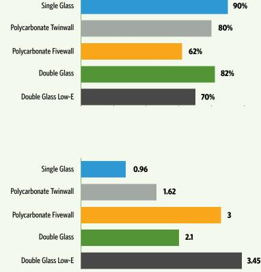
MULTIPLE LAYERS WITH AIR GAPS REDUCE CONVECTION AND CONDUCTION.
